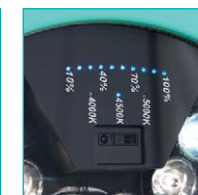
Adjustable light intensity with touchless infrared sensor
